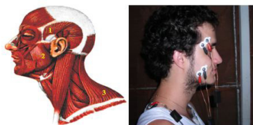
Figure 1 - Placement of surface electrodes. 1) Temporalis anterior. 2) Masseter 3) Trapezius.
